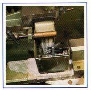
Finishing of the tip is also done with a grinder. The exact shape is given with a guide sliding on a true surface.
