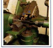
After sawing off the guide pin used as a center on the lathe, the beak is shaped by a diamond grinder for ultimate consistency.
