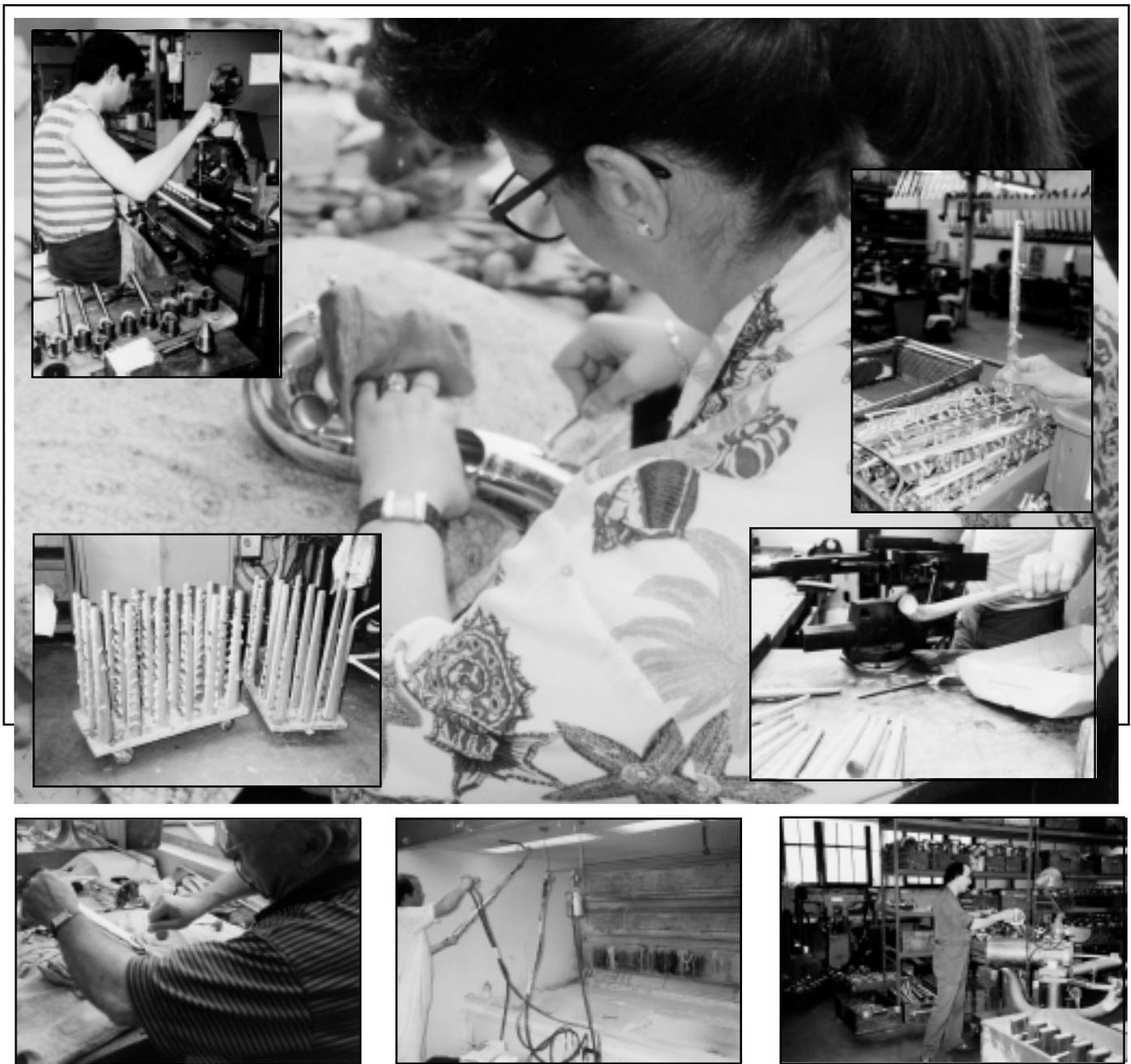
eighteen hundred saxophones each month. A combination of hand-done functions, and some that are completed by automated machinery, are used here.
